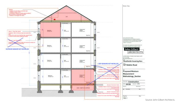
Figure 14. Section of the building showing the rooms where the interstitial condensation sensors were installed.
